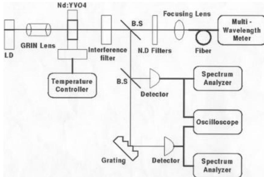
FIG. 1. The experimental setup of a diode-pumped microchip Nd:YVO<sub>4</sub> laser.
